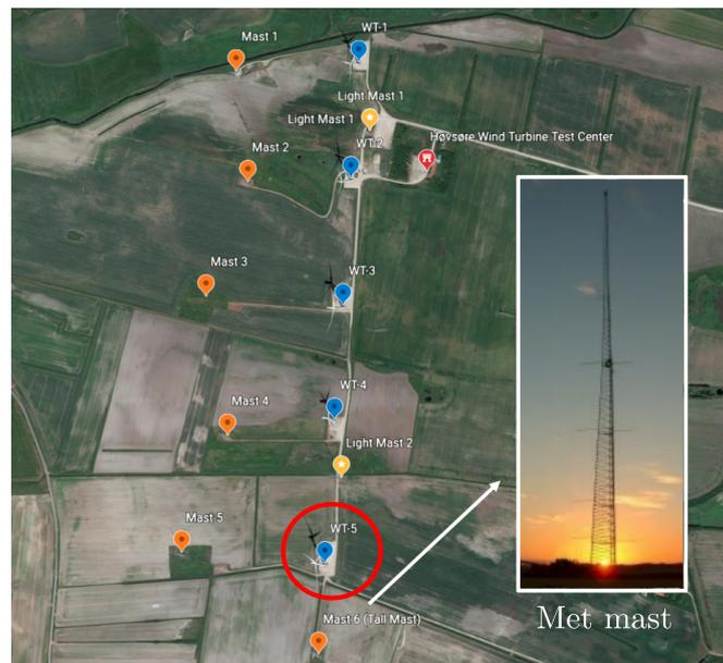
**Figure 11:** Schematic of the Høvsøre site when looking from the top, showing the wind turbines and instrumentation installed in the test site. The wind turbine considered in this work is encircled by the red circle. Experimental data was collected from a 116.5 m met mast shown in a white box. A screenshot from Google Earth satellite imagery of Høvsøre, Denmark. Met masts are shown by orange and yellow pins, whereas wind turbines are depicted by blue pins.
