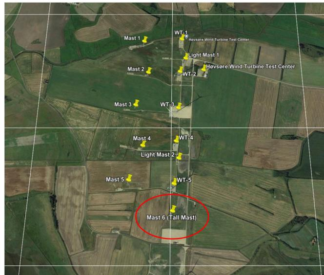
**Figure 13:** A screenshot from Google Earth satellite imagery of Høvsøre, Denmark, with wind turbines and experimental means indicated by yellow pins. The Høvsøre mast is encircled by a red ellipse. The white solid boxes indicate the boundaries of the finest WRF grid projected onto the test site ( $\Delta x = \Delta y = 1$  km).
