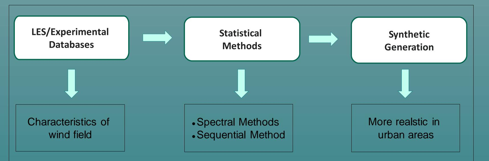
understand the characteristic of wind fields. This database is used to provide statistical information required by numerical generation methods such those based in spectral representations of the wind velocity field such as the one proposed by Mann [2], or those based on time series techniques such the sequential method proposed by Krenk [3].
